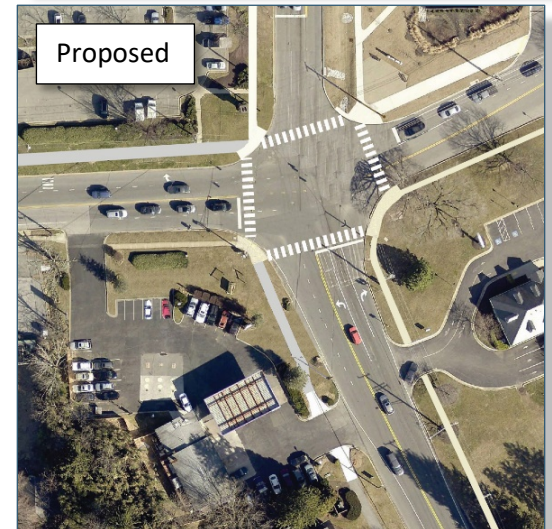
Figure 4. Revised intersection at MD 108 and MD 650 with marked crosswalks, new sidepaths and sidewalks, an increased turning radius in the northeast corner and fewer driveways at the filling station in the southeast corner.
