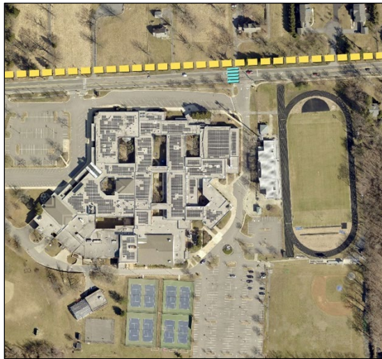
Figure 5. The recommended shared-use path is shown in yellow along the north side of MD 108. A new crosswalk and walk signal is recommended at the existing traffic signal at the high school's eastern entrance.
