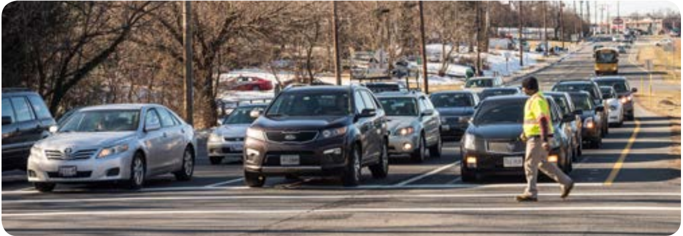
Man walks across four lanes of vehicle traffic at the intersection of Georgia Avenue and Hewitt Avenue. Roadways like this do not support Vision Zero principles: wide lanes encourage speeding; lack of pedestrian islands and of high visibility crosswalks, narrow sidewalks and absence of bike facilities fail to provide adequate separation between different road users.
