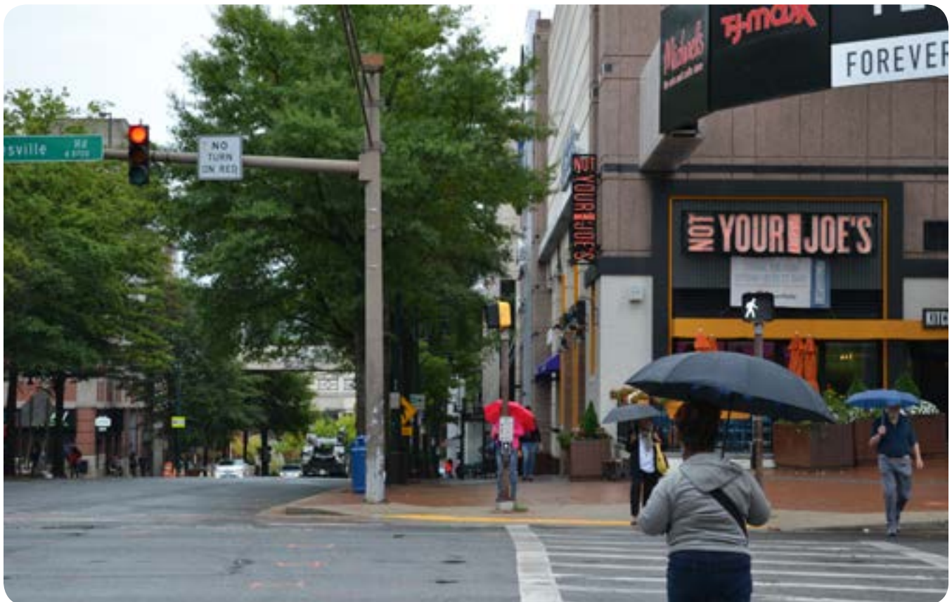
LPIs allow pedestrians to begin crossing while vehicle traffic still has a red light, enabling them to reach the middle of the intersection and to be more visible to turning drivers.
