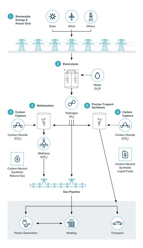
In the study, power-to-X refers to electrolysis that converts surplus electricity into hydrogen, which then is combined with carbon dioxide, captured either through direct air capture powered by carbon-free electricity, or from biorefineries to produce methane gas (power-to-gas). The Fischer-Tropsch synthesis process can also be used to create synthetic liquid fuels to replace conventional oil based transport fuels (power-to-liquids).
