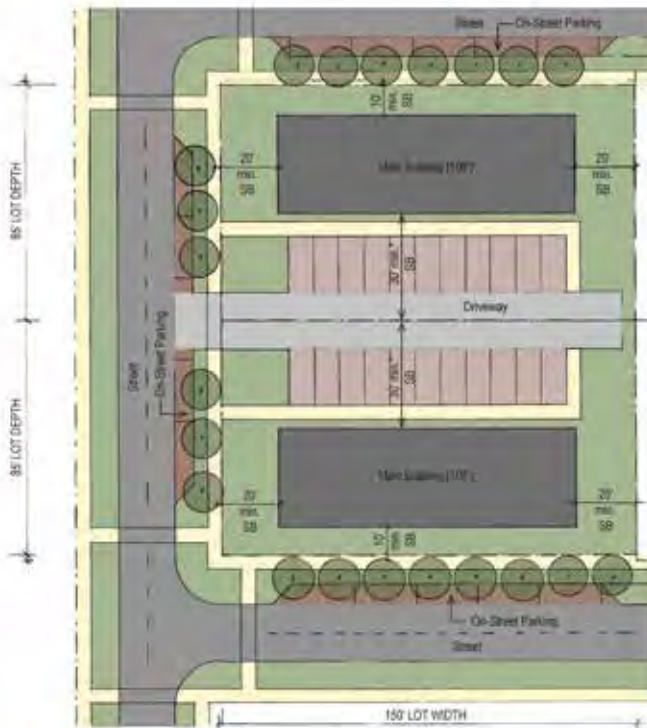
Garden Apartment Low-rise (15 unit)
