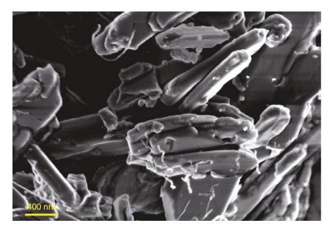
One of the research areas for the Consortium is the use of new carbon materials in lead batteries. Carbon additives, such as Exide Technologies' carbon nanotubes (CNT)s pictured above in the active mass of a positive electrode in a lead battery, open new avenues for improvements in cycle life and DCA.
