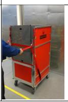
The container secured and ready for transportation by the straps and single snap buckle
