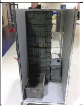
The loose stack at the rear can be stabilised by placing up to 3 upturned trays at the right hand side of the rear stack
