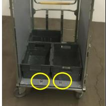
The tray stacks are located by means of the lugs shown
