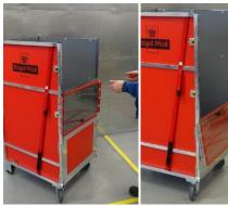
The top 2 sections can be folded down and up to aid filling and emptying the container.
